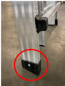
2. Drill a 10 mm diameter hole in the center of the upright at a height of 100 mm.
