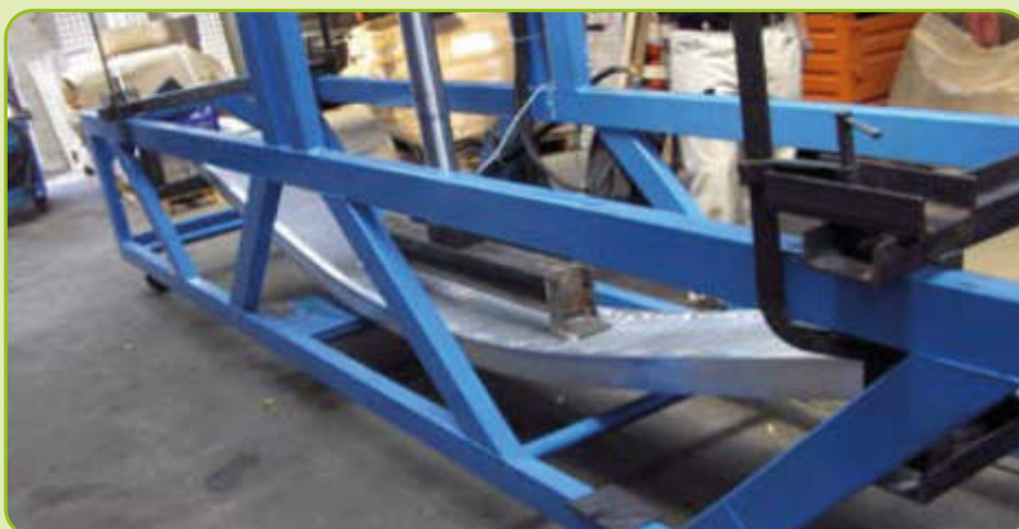
Ramp subject to breakage.
